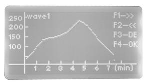
② Following we provide eight different waves, please choose one according to your request. Press the F1/F2 to choose different wave, press F3 to look into different wave parameter, press 4 to confirm the wave you chose.
