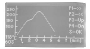
Press F1/F2 button, ahead/ backwards select different time. Press F3/F4 button ,up/down to select different temperature, Press "s" button to save.
