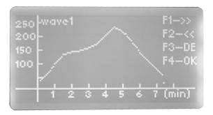
Press "F3" button again, can see parameter about you choose the temperature wave: **Select**: soldering paste sort, soldering temperature, time etc. example:
